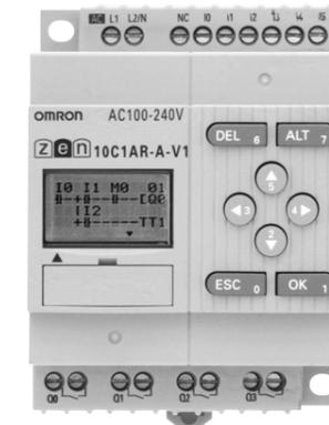
ZEN-10C1AR-A-V1 (AC type, relay outputs)
